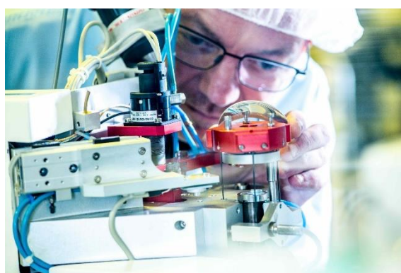
Adjustment of equipment for high volume lens replication [photo credit Anteryon]
